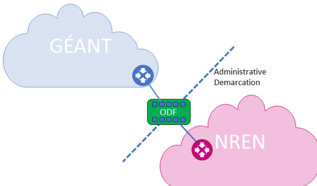
**Figure 5: Illustration of the management demarcation point**
