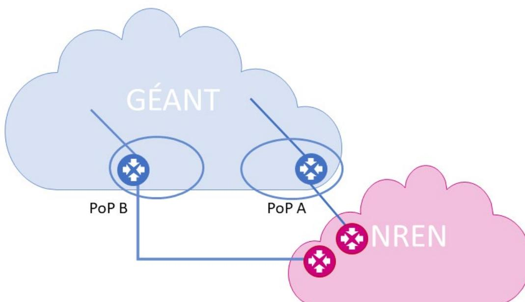
**Figure 4: Example of load sharing on multiple PoPs**
